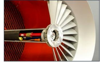
The spin vanes and other components of the nose ensure flame stability and optimum shape.
