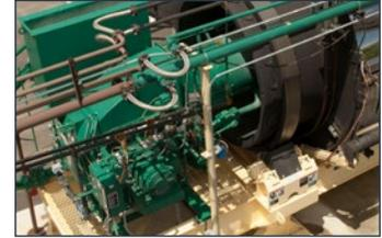
The Phoenix Talon uses less electric power due to the variable frequency drive used to control its combustion air blower and low body pressure.
